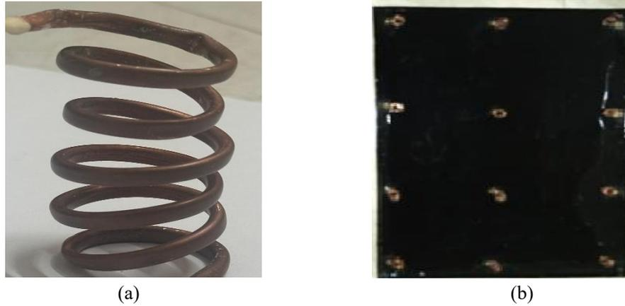
**Fig 1. (a)** Contraction of a single coil fin **(b)** Coil shaped fins placed on absorber plate
